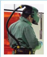
The filter and fan are mounted on the waist belt of this battery powered welding kit. It delivers filtered air to the welder from the flexible hose at the back of the unit.
