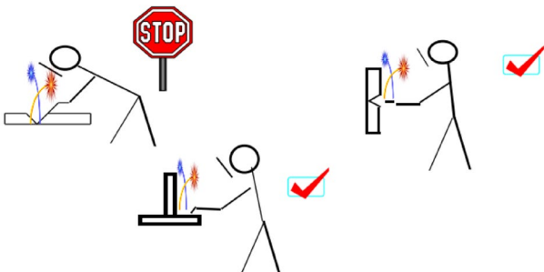
Figure 7.3: The welder's head should not enter the visible fume plume.
